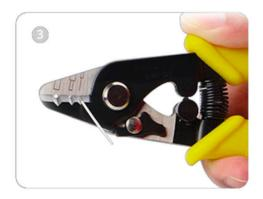
• Strip the 250µm coating(With the smallest hole)
