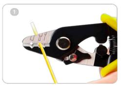
• Strip the 900µm buffer coating(With the second hole)
